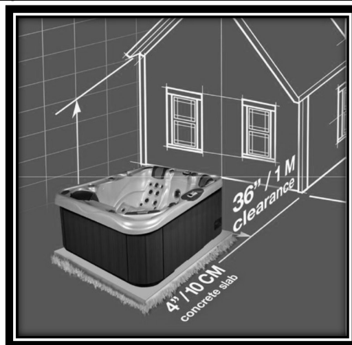
Figure 1 - Space Required (Clearance) and Support
