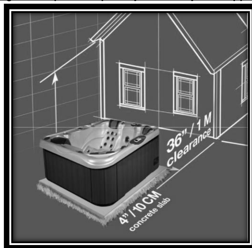
Figure 1 - Space Required (Clearance) and Support
